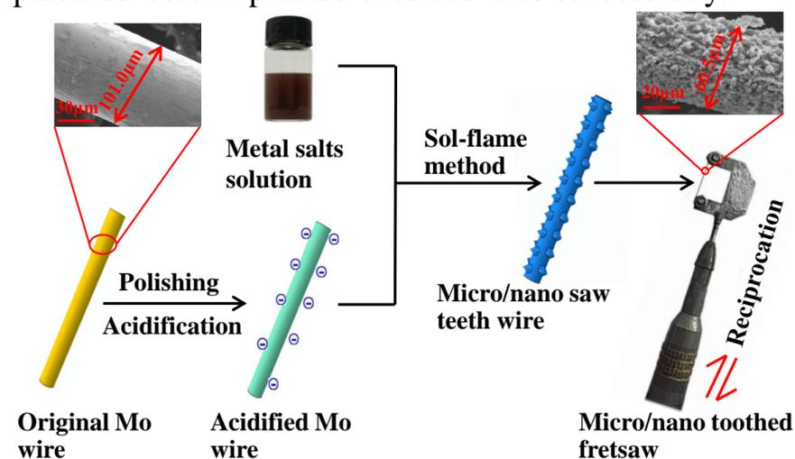
Figure 1. The preparation process of micro/nano toothed fretsaw
