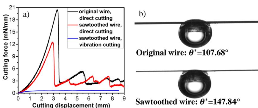
Figure 2. cutting forces-displacement curve (a) and apparent angle (b) of original wire and sawtoothed wire
