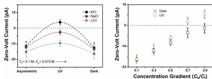
A bioinspired photo-driven ion pump based on single PET conical nanochannels is developed. The pumping process behaving as an inversion of zero-volt current can be realized by applying UV irradiation from the large opening. Enhanced electrostatic interaction between the ions and the charged groups on the inner wall is the key reason.
