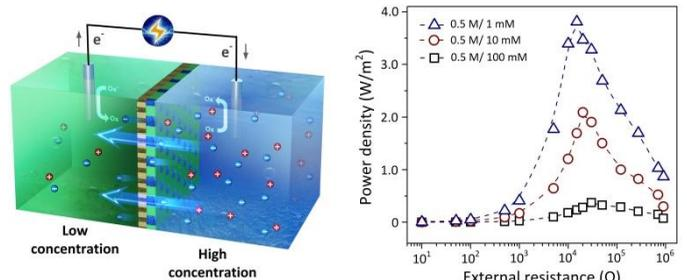
To expand to new avenues and stay economically attractive, membrane development must constantly strive for higher permeability and seek new and better selectivity. Next, we developed a block copolymer based ultrathin Janus membrane with excellent anion selectivity. The sub-micrometer scale thickness ( $\approx 500 \text{ nm}$ ) of the system provides very low ion resistance and high permeability, which enable an enhancement in the output density to approximately  $3.9 \text{ W/m}^2$ .
