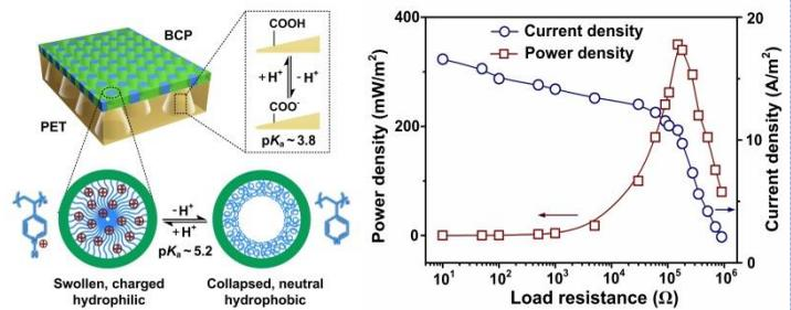
We first develop a proof-of-concept asymmetric bipolar heterogeneous membrane system with ultrahigh ion rectification. The system can achieve a power density approximately  $0.35 \text{ W/m}^2$  by mixing river water and sea water, which outperforms many commercial ion exchange membranes.
