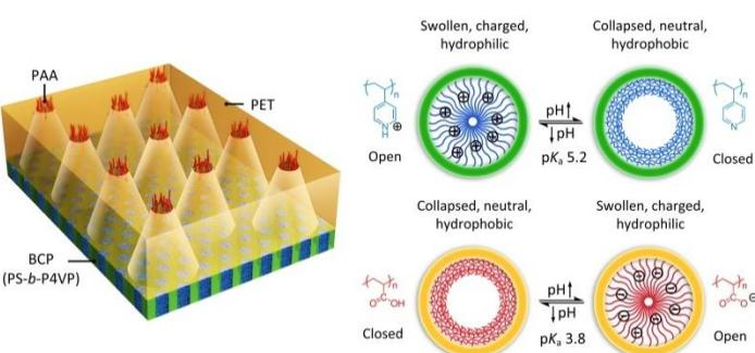
We then develop a bioinspired heterogeneous ion pump membrane with unidirectional selective ion pumping and efficient ion gating behaviors. Great controllability on the gating ability can be realized by tailoring the asymmetric pore distribution. These studies are an important step toward a procedure that mimics smart transport in life pump systems.
