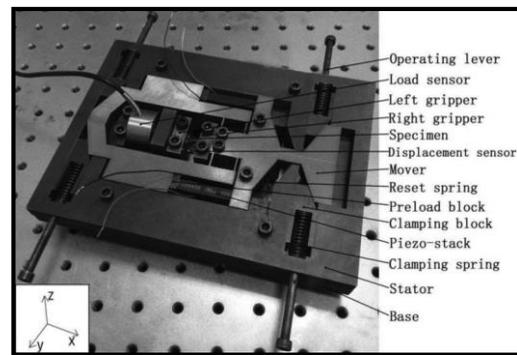
Fig. 1. Structure of the device.
