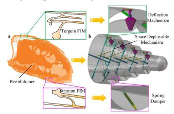
We take inspiration from variant structure of honeybee's abdomen to design a morphing nose cone of aerospace vehicle. Mechanical design and simulation analysis are conducted to optimize the geometric structural parameters of the morphing nose cone.
