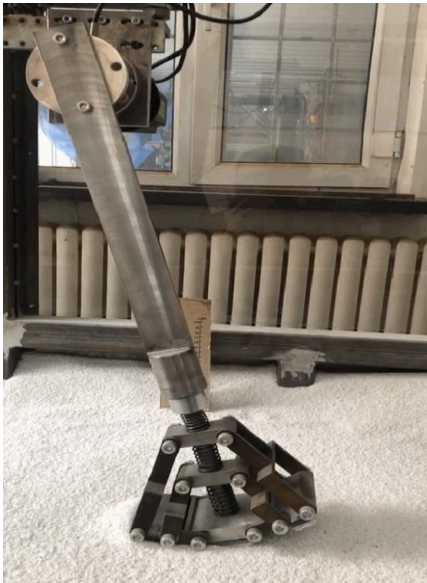
Test for bionic foot travelling on sand
